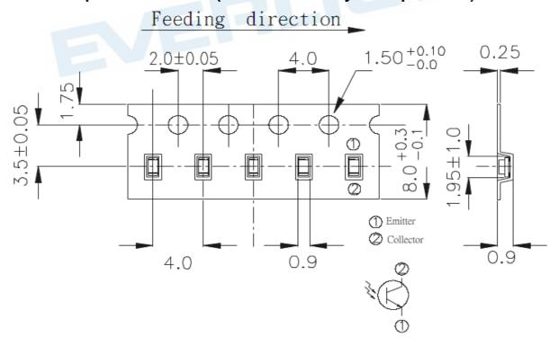
**Note:** The tolerances unless mentioned are  $\pm 0.1$ , unit=mm
