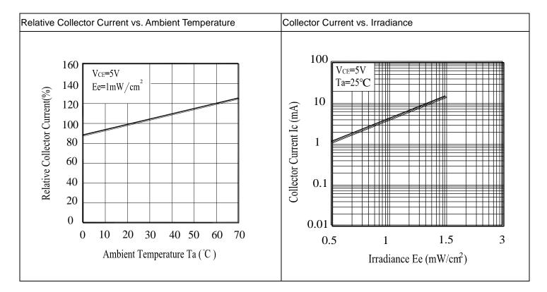
DATASHEET 5mm Phototransistor PT333-3C
