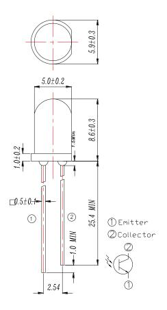
Note: Tolerances unless dimensions ±0.25mm
