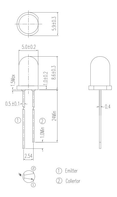
Note: Tolerances unless dimensions ±0.25mm
