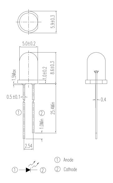
Note: Tolerances unless dimensions ±0.25mm
