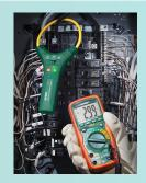
Expand your meter's capabilities to measure AC Current up to 3000A. Fit most MultiMeters or Clamp Meters with standard shrouded banana plug sockets. Flexible clamp jaw easily wraps around bus bars and cable bundles where standard clamp adaptors and meters can't. The thin 7.5mm cable diameter easily fits into tight spaces. Choose between a 10" (25.4cm) or 18" (45.7cm) clamp cable lenoth.
