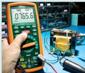
Measure the insulation resistance of transformer windings
