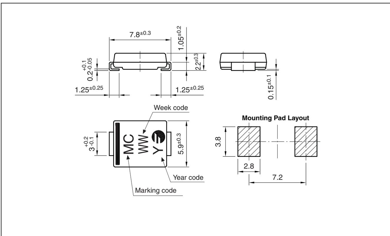
**3.0 Amp. Surface Mount Glass Passivated Rectifier**
