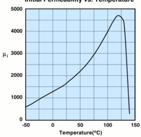
Measured on a 17/10/6mm toroid at 100kHz.
