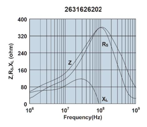
Impedance, reactance, and resistance vs. frequency.
