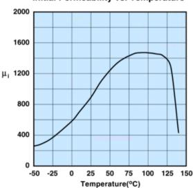
Measured on a 17/10/6mm toroid at 100kHz.
