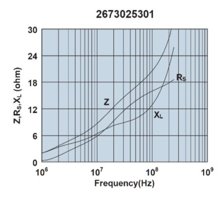
Impedance, reactance, and resistance vs. frequency.
