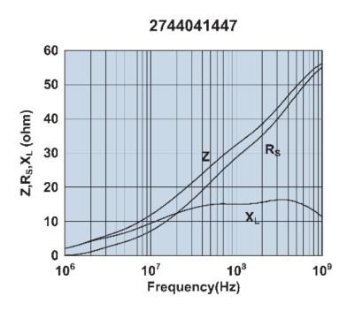
Impedance, reactance, and resistance vs. frequency.
