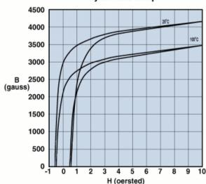
Measured on a 17/10/6mm toroid at 10kHz.
