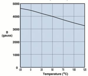
Measured on a 17/10/6mm toroid at 10kHz. and H=10 oersted.
