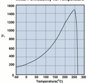
Measured on a 17/10/6mm toroid at 100kHz.
