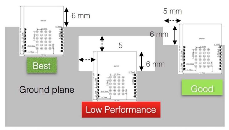
1.Module extends 6 mm from edge or ground plane of the host PCB board.
