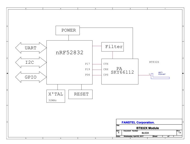
A firmware configuration example to control Skyworks SKY66112 power amplifier is below. This firmware file, SKY66112\_PAconfig.txt can be downloaded from <a href="http://www.fanstel.com/download-document/">http://www.fanstel.com/download-document/</a>.
