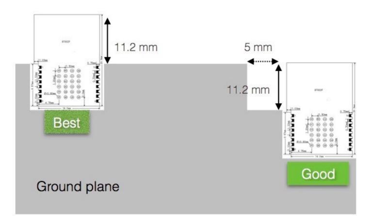
1.BT832F module extends 11.2 mm from edge or ground plane of the host PCB board.
