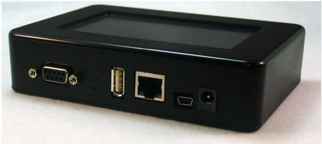
uEZGUI-2478-43WQS with uEZGUI-EXP1 mounted in OEM Housing
