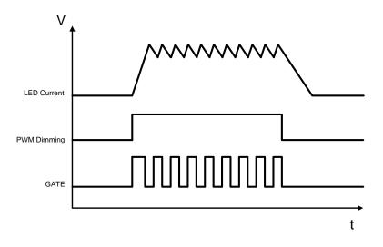
The rising and falling edges are limited by the current slew rate in the inductor. The first switching cycle is terminated upon reaching the 250mV ( $V_{DIM} \cdot 0.167$ ) level at CS. The circuit is further reaching its steady-state within 1 switching cycles regardless of the switching frequency.
