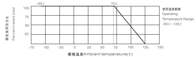
\* 當電阻使用的環境温度超過70℃時,其額定負荷(額定功率或額定電流)按上述曲綫下降。 For resistors operated in ambient over 70℃, rated load (power rating or current rating) shall be derated in accordance with above figure.
