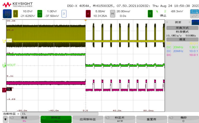
短路保护, V_{IN} = 12V , V_{OUT} = 3.3V 3A to Short
