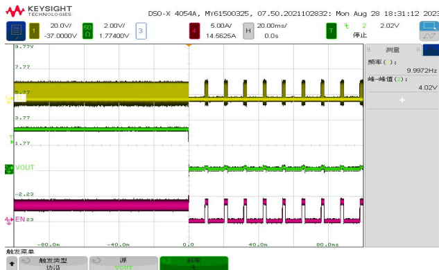
短路保护, V_{IN} = 12V , V_{OUT} = 3.3V 3A to Short
