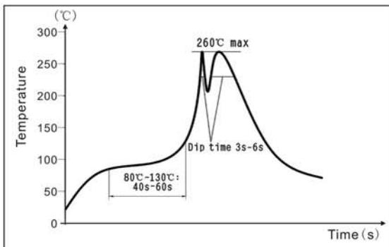
● 推薦的焊膏類型 Recommended solder alloy: 96.5Sn/3.0Ag/0.5Cu
