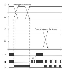
Legend: T2 = 1÷60 s If the wrong phase rotation sequence is detected at the input terminals of the device, the relay will be switched off immediately. The red LED will be on to indicate a phase sequence error. When the correct phase sequence returns, the relay will be switched on with a delay of T2. The green LED [R] will flash until the relay is switched switch (time T2).
