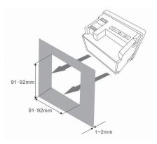
Insert the multimeter from the front of the panel with all wires disconnected and press it against the surface of the panel.
