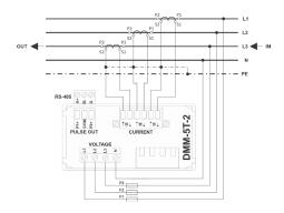
3P4W system - 3-phase, 4-wire network, semi-indirect measurement
