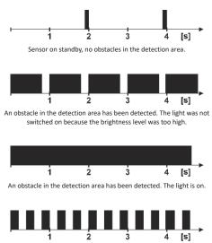
Signalling that the acceptable temperature inside the sensor is exceeded. Sensor operation is blocked until the fault has been removed.
