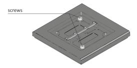
Disconnect the button stand from the frame and electronics.
