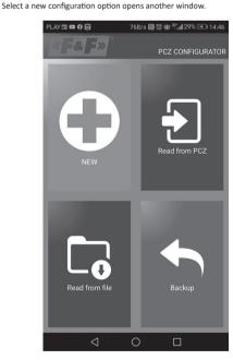
The function window allows to edit program as well as to load and save configuration to a PCZ controller. It appears automatically when we bring the phone closer to the controller, or when we create a new configuration. In the upper part of the screen the application displays a frame with following information:
