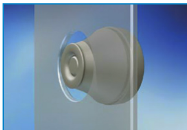
Push the grommet into the hole.
