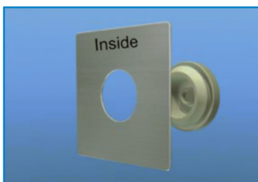
Push the grommet into the hole.
