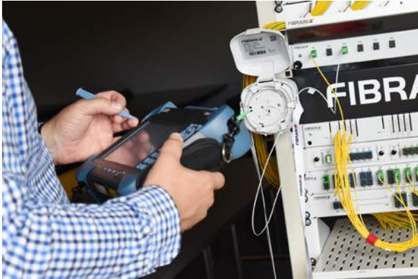
Pic 5. Mounting the FIBRAIN starter cube on a magnet and to a fiber optic cabinet
