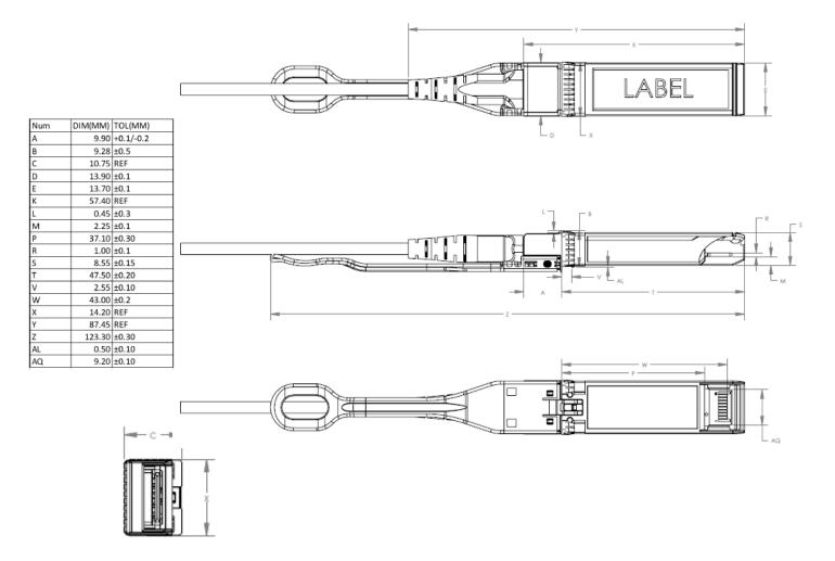
Figure 2. FCBG125SD1Cxx Mechanical Dimensions.
