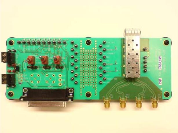
Finisar's FDB-1027 Evaluation Board is the perfect vehicle for testing and evaluating SFP/SFP+ optical transceivers.
