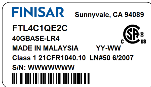
Figure 3 – FTL4C1QE2C production label
