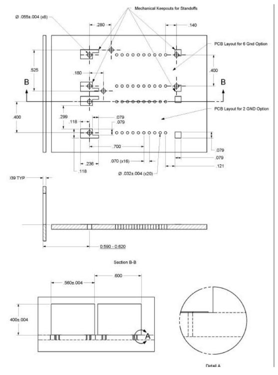
Minimum Recommended Module-to-Module Spacing is 0.6 inches
