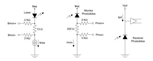
Analog monitoring function connections.
