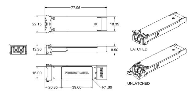
XFP Transceiver (dimensions are in mm)
