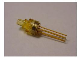
The HFD3141-203 use a high-performance InGaAs PIN photo-detector packaged with a transimpedance amplifier designed to meet performance requirements for data rates up to 4.25Gbps data communication over single-mode optical fiber at 1200nm to 1600nm. Applications include Ethernet, Fiber Channel and ATM protocols. The PIN is RoHS compliant per Directive 2011/65/EU<sup>1</sup>.
