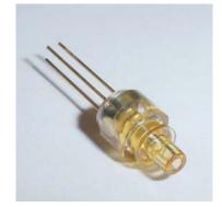
This product is a high-performance 850nm VCSELs (Vertical Cavity Surface-Emitting Lasers) designed for high-speed data communications and packaged with a custom designed power monitor diode. The power monitor diode can be used with appropriate feedback control circuitry to set a maximum power level for the VCSEL. These combined features simplify design for high data rate communication and eye safety.
