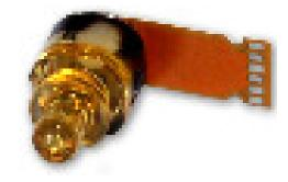
The HFE7192-6x1 uses a high-performance Vertical Cavity Surface Emitting Laser (VCSEL) designed to meet performance requirements for 1/2/4/8 Gbps data communication over multimode optical fiber for the ANSI X2.T11 Fibre Channel protocols. The optical assembly is designed to interface either 50mm
