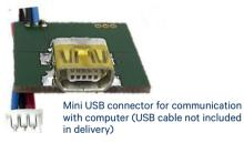
Serial interface connector to SiPM Module
