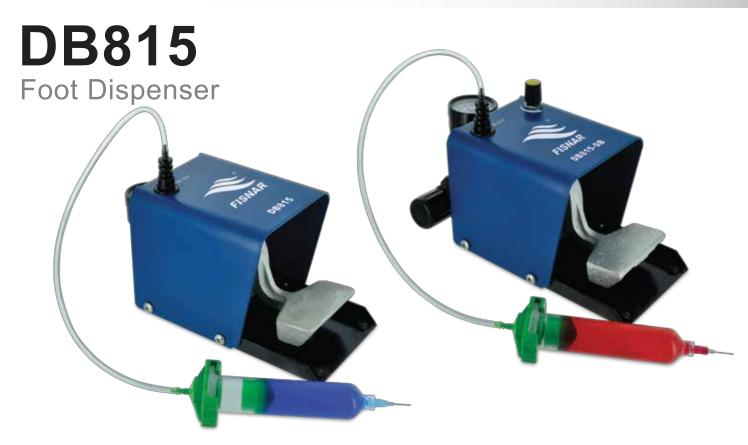
A basic air-powered system, floor mounted and foot actuated. Includes a three-way air valve and built in air regulator, ideal for non-critical dispensing operations. As long as the foot pedal is depressed, fluid will be dispensed. The unit is suitable for all types of fluids. The model with suck-back option ensures that low viscosity liquids do not drip.
