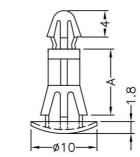
HOLE IN CHASSIS Ø5.5 CHASSIS THICKNESS 1.2~1.8
