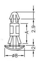
HOLE IN CHASSIS Ø4.0 CHASSIS THICKNESS 0.8~1.6
