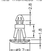
HOLE IN CHASSIS Ø4.8 CHASSIS THICKNESS 0.8~2.0
