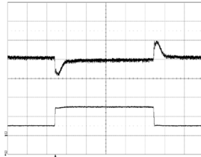
Output voltage response to load current step- change (9.5 – 28.5 – 9.5 A) at: T_{ref} = +25^{\circ}\text{C} , V_1 = 53\text{ V} , C_o = 3.8\text{ mF}
