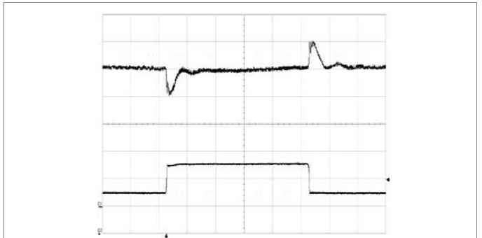
Output voltage response to load current step- change (10 - 30 - 10 A) at: T_{ref} = +25^{\circ}C, V_I = 53 V, C_o = 4 mF
