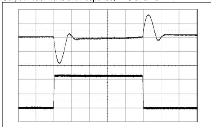
Output voltage response to load current step-change (6.25-18.75-6.25 A) at: T_{P1} = +25\text{ }^{\circ}\text{C} , V_I = 12\text{ V} , V_O = 1.0\text{ V} di/dt = 2\text{ A}/\mu\text{s} , f_{sw} = 320\text{ kHz} , C_O = 470\text{ }\mu\text{F}/10\text{ m}\Omega DLC and no NLR
