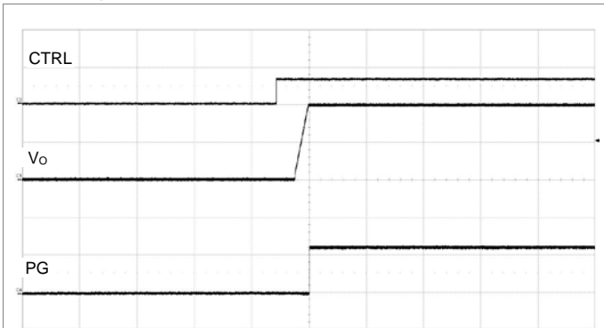
Output enabled by CTRL pin. V_i = 12\text{ V} , I_o = 80\text{ A} . TON\_DELAY = TON\_RISE = 5\text{ ms} , POWER\_GOOD\_DELAY = 1\text{ ms} . Scale from top: 5, 0.5, 2 V/div, 20 ms/div.
