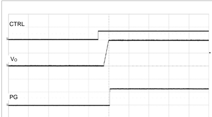
Output enabled by CTRL pin. V_i = 12\text{ V} , I_o = 40\text{ A} . TON\_DELAY = TON\_RISE = 5\text{ ms} , POWER\_GOOD\_DELAY = 1\text{ ms} . Scale from top: 5, 0.5, 2 V/div, 20 ms/div.
