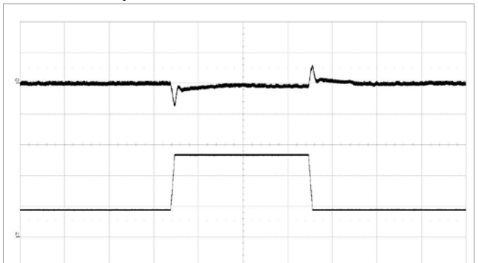
Output voltage response to load current step change (25%–75%–25%) at V_I = 12\text{ V} , C_{OUT} = 8 \times 330\text{ }\mu\text{F}/10\text{ m}\Omega + 20 \times 100\text{ }\mu\text{F} , di/dt = 2\text{ A}/\mu\text{s} , ACSR\text{ Gain} = 219 and ASCR\text{ Residual} = 82 . Scale from top: 50 mV/div, 20 A/div, 200 \mu\text{s} /div. Note: Sense pins are connected to load.
