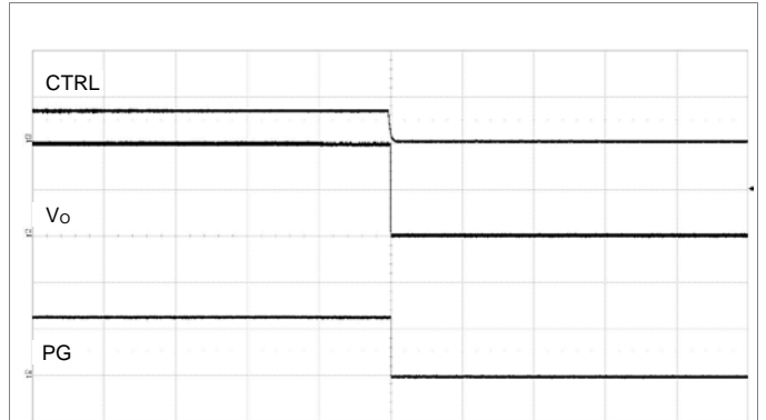
Output disabled by CTRL pin. V_i = 12\text{ V} , I_o = 40\text{ A} . Scale from top: 5, 0.5, 2 V/div, 20 ms/div.
