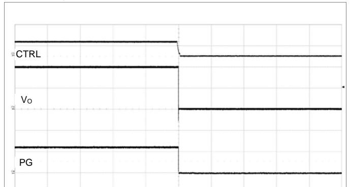
Output disabled by CTRL pin. V_i = 12\text{ V} , I_o = 80\text{ A} . Scale from top: 5, 0.5, 2 V/div, 20 ms/div.
