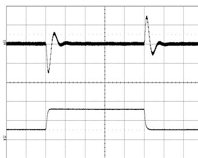
Output voltage response to load current step- change (2.5-7.5-2.5 A) at: T_{ref} = +25^{\circ}\text{C} , V_1 = 53\text{ V} . Top trace: output voltage (200mV/div.). Bottom trace: load current (5A/div.). Time scale: (0.1ms/div.).
