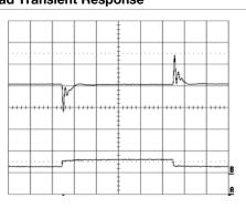
Output voltage response to load current step- Top trace: output voltage (100mV/div.).
