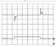
Output voltage response to load current step- Top trace: output voltage (100mV/div.).
