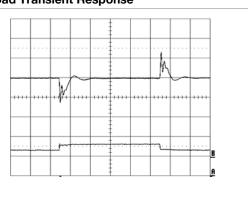
Output voltage response to load current step- Top trace: output voltage (100mV/div.). change (3-6-3 A) at: Bottom trace: load current (10 A/div.).  $T_{ret} = +25^{\circ}\text{C}, \ V_{l} = 3.3 \ \text{V}.$  Time scale: 0.1 ms/div.
