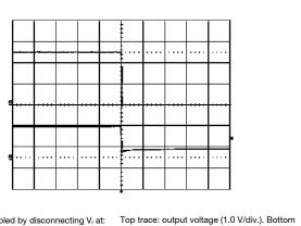
Shut-down enabled by disconnecting V $_{\rm l}$  at:  $T_{\rm ref}=+25\,^{\circ}\text{C},\ l_{O}=6$  A resistive load, V $_{\rm l}=3.3$  V.
