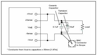
Output ripple and noise test setup
