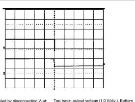
Shut-down enabled by disconnecting V<sub>I</sub> at:  $T_{ref} = +25^{\circ}C$ ,  $I_{O} = 6$  A resistive load,  $V_{I} = 3.3$  V.
