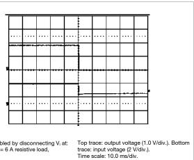
Shut-down enabled by disconnecting V<sub>I</sub> at:  $T_{\text{ref}} = +25^{\circ}\text{C}$ , I<sub>O</sub> = 6 A resistive load, V<sub>I</sub> = 3.3 V.
