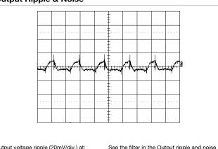
Output voltage ripple (20mV/div.) at:  $T_{ref} = +25^{\circ}C$ ,  $I_{O} = 6$  A resistive load,  $V_{I} = 3.3$  V. Time scale: 1  $\mu$ s/div.
