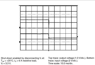
Top trace: output voltage (1.0 V/div.). Bottom trace: input voltage (2 V/div.). Time scale: 10.0 ms/div.
