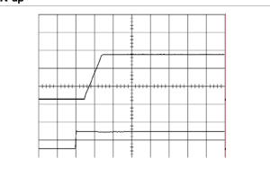
Start-up enabled by connecting V<sub>I</sub> at:  $T_{ref} = +25^{\circ}C$ ,  $I_{O} = 15$  A resistive load,  $V_{I} = 5.0$  V.
