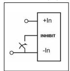
The products are fitted with a remote control function referenced to the primary negative input connection (- In), positive logic. The INHIBIT function allows the regulator to be turned on/off by an external device like a semiconductor or mechanical switch. The INHIBIT pin has an internal pull up resistor to + In.
