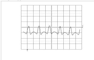
Output voltage ripple (20mV/div.) at:  $T_{ref}$  = +25°C,  $I_O$  = 15 A resistive load,  $V_I$  = 5.0 V. Time scale: 2 µs/div.
