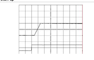
Start-up enabled by connecting V<sub>I</sub> at:  $T_{ref} = +25^{\circ}C$ ,  $I_{O} = 15$  A resistive load,  $V_{I} = 5.0$  V.
