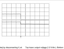
Shut-down enabled by disconnecting V<sub>i</sub> at:  $T_{ref}$  = +25°C, I<sub>O</sub> = 15 A resistive load, V<sub>i</sub> = 5.0 V.
