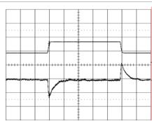
Output voltage response to load current step- Top trace: output voltage (100mV/div.). change (7-15-7 A) at: Bottom trace: load current (10 A/div.).  $T_{ref} = +25^{\circ}\text{C}, \ V_i = 5.0 \text{ V}.$  Time scale: 0.1 ms/div..
