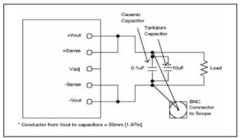
Output ripple and noise test setup
