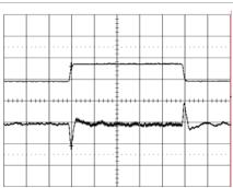
Output voltage response to load current step- Top trace: output voltage (100mV/div.). change (7-15-7 A) at: Bottom trace: load current (10 A/div.).  $T_{ref} = +25^{\circ}\text{C}, \ V_i = 5.0 \text{ V}.$  Time scale: 0.1 ms/div..
