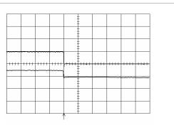
Shut-down enabled by disconnecting V<sub>i</sub> at:  $T_{ref}$  = +25°C, I<sub>O</sub> = 15 A resistive load, V<sub>i</sub> = 5.0 V.
