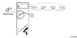
To return to autorange, press  $\ \ \ \ \ \ \ \ \ \$  for 1 second or turn the rotary switch.
