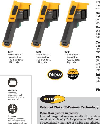
stand, which is why Fluke pioneered IR-Fusion, a revolutionary marriage of visible and infrared images never before seen in commercial or industrial thermal imagers. Automatically capturing a visible image with every infrared image allows to you always know exactly what you're looking at.
