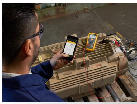
Store and share data using the Fluke 1587 FC with Fluke Connect Measurements App.
